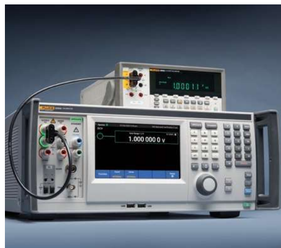
The 5550A calibrates the most popular 5.5-digit desktop multimeters.
